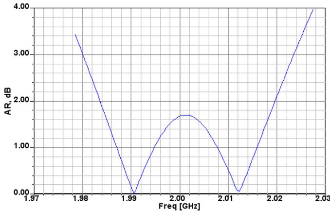
Fig.3. Axial Ratio versus frequency,  $\epsilon_r=2.2$ ,  $h=1.5$  mm
