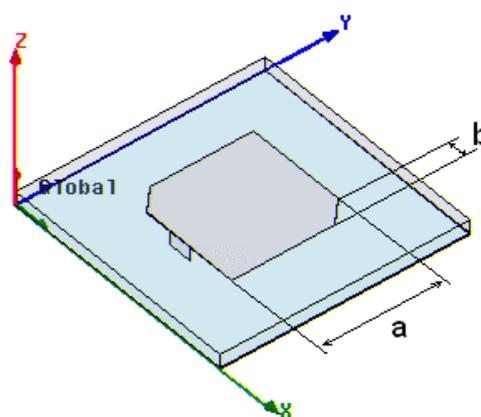
Fig.1. Circularly polarized microstrip antenna with truncated corners
