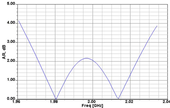
Fig.4. Axial Ratio versus frequency,  $\epsilon_r=2.2$ ,  $h=2$  mm
