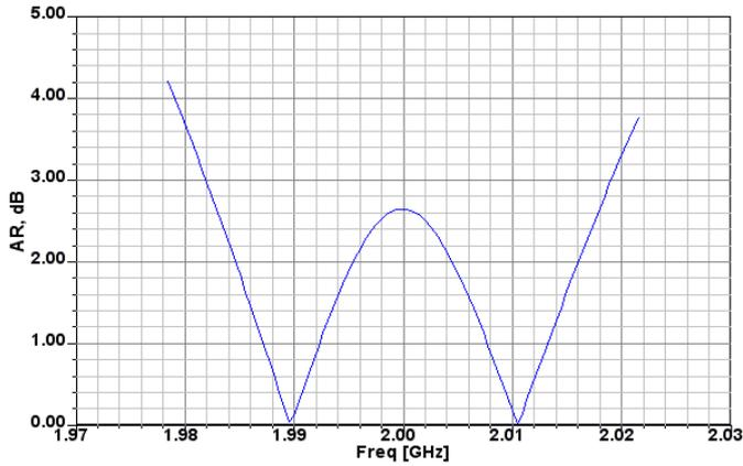
Fig.2. Axial Ratio versus frequency,  $\epsilon_r=2.2$ ,  $h=1.1$  mm
