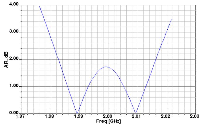
Fig.5. Axial Ratio versus frequency,  $\epsilon_r=2.2$ ,  $h=1.4$  mm
