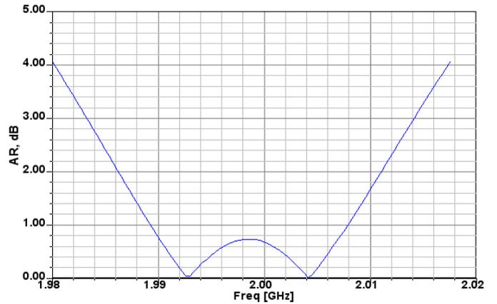
Fig.6. Axial Ratio versus frequency,  $\epsilon_r=5$ ,  $h=1.4$  mm
