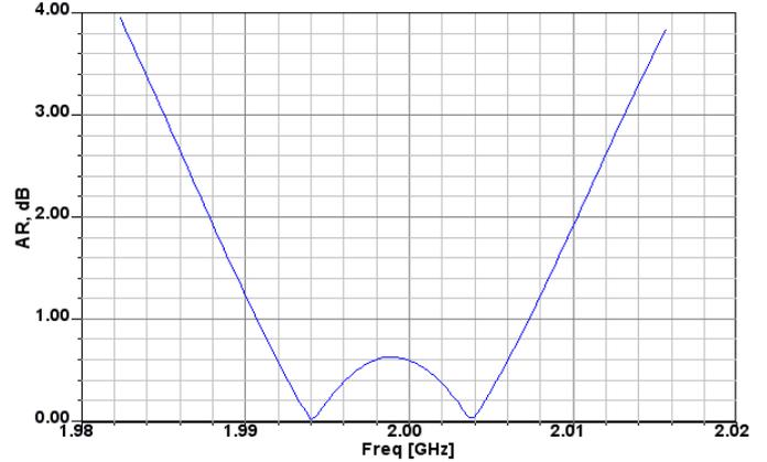
Fig.7. Axial Ratio versus frequency,  $\epsilon_r=7.5$ ,  $h=1.4$  mm
