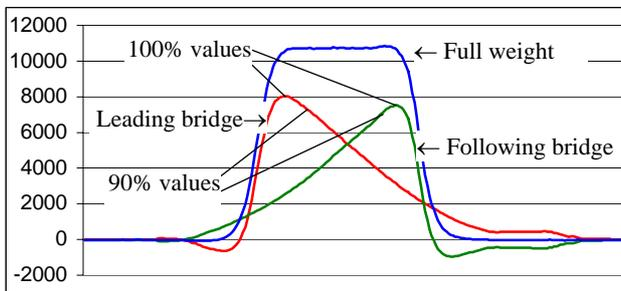
Fig. 3. Primary signal for D2 wheel (left movement).
