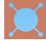
Fig. 3. New hole shape for bolts in bolted busbar connections
