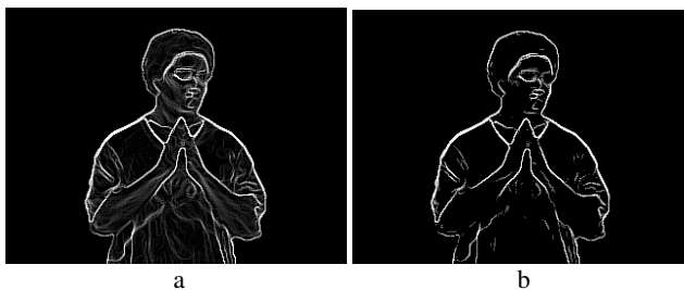
Fig. 7a. Contour image (contours were extracted with Corel Photo Paint 10, Edge detection); b. Same image, after filtration.
