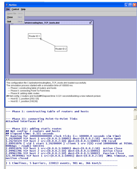
Fig. 1. Sample graphical user interface (GUI) application showing results of the SSFNet network simulation.
