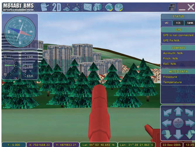
Fig. 6. BMS user interface in the 3D View
