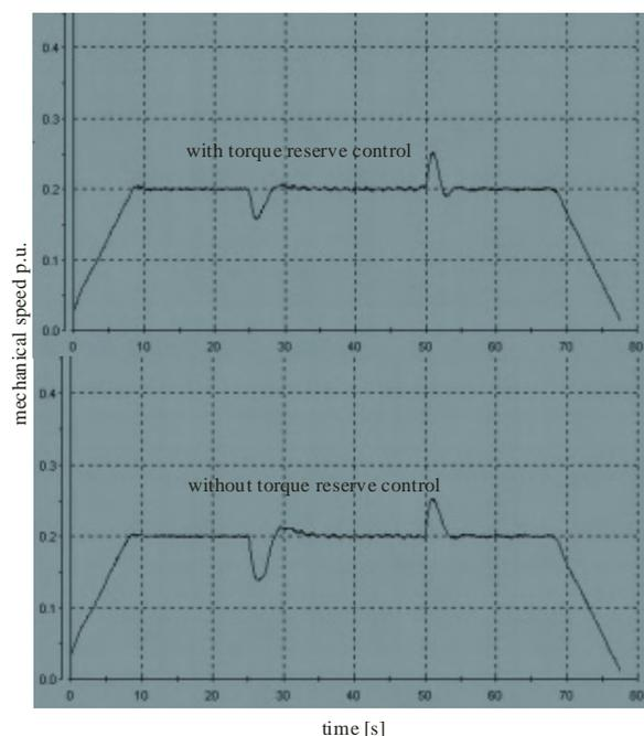
Fig. 5. Graphics of mechanical speed for a step change of load torque.
