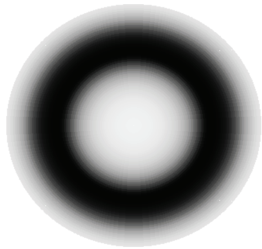
Fig.7. Thickness distribution over the substrate holder
