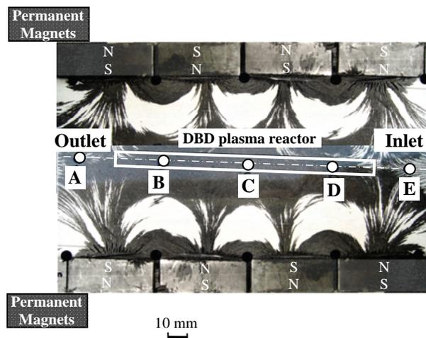
Fig. 5. *MDBD* plasma reactor with two co-axial discharge tube – graph of the magnetic flux density of an open magnetic system with alternating poles of the permanent magnets arranged bilaterally to the discharge tube in one layer.
