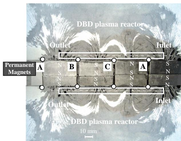
Fig. 4. *MDBD* plasma reactor with two co-axial discharge tube – graph of the magnetic flux density of an open magnetic system with four alternating poles of the permanent magnets arranged in two layers.
