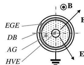
Fig. 2. Co-axial types (tube in tube) of a magnetron DBD plasma reactor with crossed magnetic **B** and radial electric fields **E**. HVE and EGE – high-voltage electrode and earth-grounding electrode; DB – dielectric barrier; AG – air (discharge) gap.
