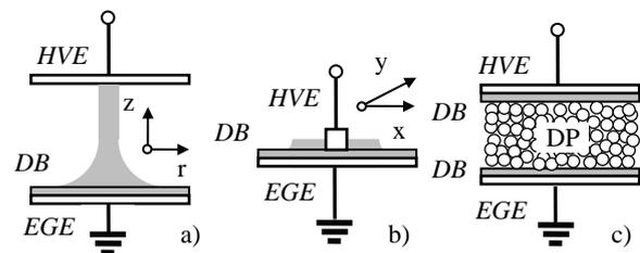
Fig. 1. Different types of DBDs arrangements: **a** - volume DBD plasma reactor, **b** - surface DBD plasma reactor and **c** - packed bed DBD plasma reactor.
