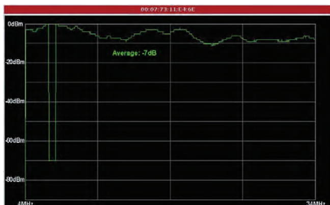
Fig. 1. – Receiver level for 2m distance
