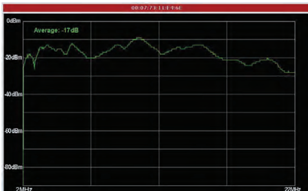
Fig. 7. – Receiver level between 2-22MHz
