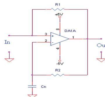
Fig.1. Voltage Negative Impedance Converter (VNIC)
