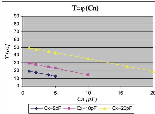
Fig.5. Summary results for the dependences  $T = \varphi(C_n)$ , through simulation
