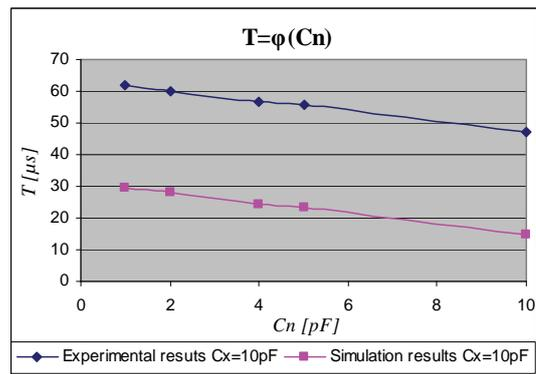
Fig.8. Dependence  $T = \varphi(C_n)$ , with  $C_x = 10$  pF
