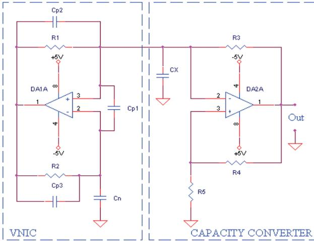
Fig.2. Capacity converter with VNIC, connected into the measured capacity  $C_x$
