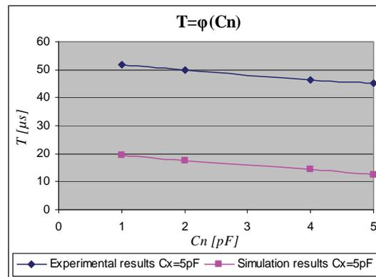
Fig.7. Dependence  $T = \varphi(C_n)$ , with  $C_x = 5$  pF
