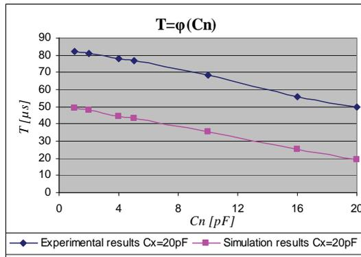
Fig.9. Dependence  $T = \varphi(C_n)$ , with  $C_x = 20$  pF
