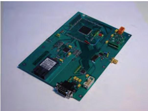
Fig. 9. BER tester model realization
