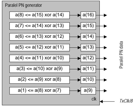
Fig. 5. Parallel PN generator in  $2^{15}-1$  case
