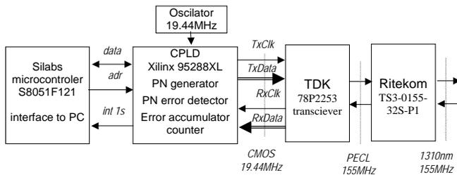
Fig. 8. BERtester model block diagram
