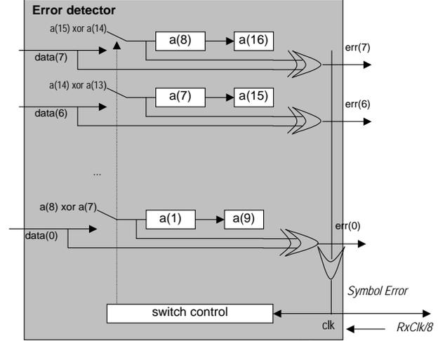
Fig. 6. Parallel Error detector in  $2^{15}-1$  case
