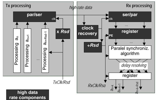
Fig. 4. General parallel signal processing architecture
