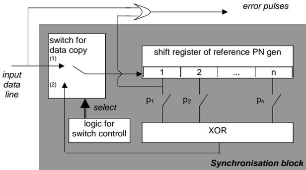
Fig. 3. Closed loop synchronization algorithm
