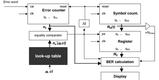
Fig. 7. Predetermined confidence BER measurement hardware
