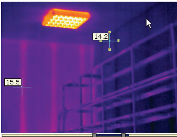
Fig.3. Temperature field in the empty storehouse
