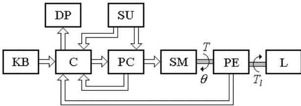
Fig. 2. Simplified block diagram of the position drive system.
