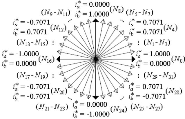
Fig. 7. Current levels when one full step is divided into 8 sub-steps.
