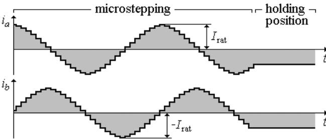
Fig. 5. Current waveforms in microstepping operation.
