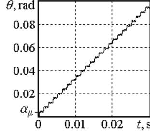
Fig. 9. Position response in microstepping operation mode when one full step is divided into 8 sub-steps.
