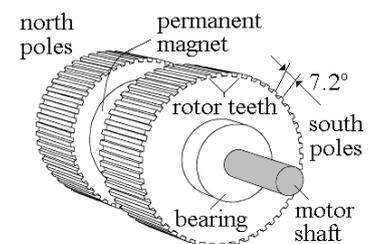
Fig. 1. The rotor of the hybrid step motor.
