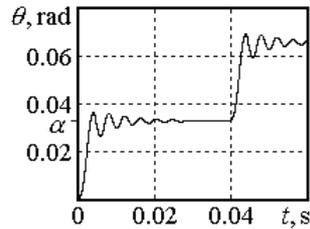
Fig. 8. Position response in full step operation mode.
