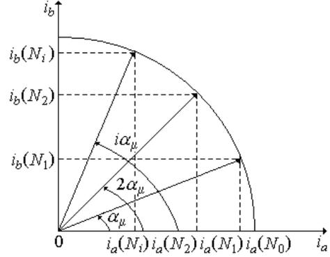
Fig. 6. Vector diagram for microstepping control.
