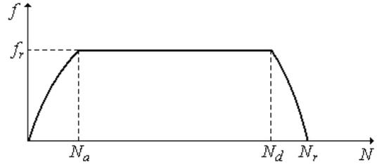
Fig. 4. Motion trajectory for a reference position cycle.
