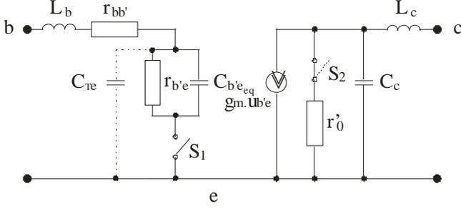
Fig. 4. High-frequency large-signal bipolar transistor model
