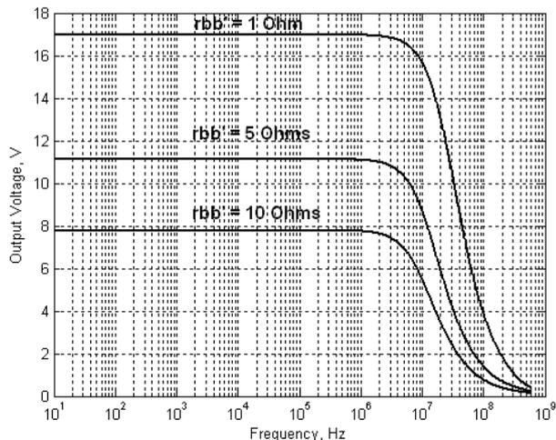
Fig. 5. Transistor output voltage as a function of frequency and base – spreading resistance
