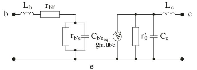
Fig. 3. Simplified high-frequency small-signal model for bipolar transistor
