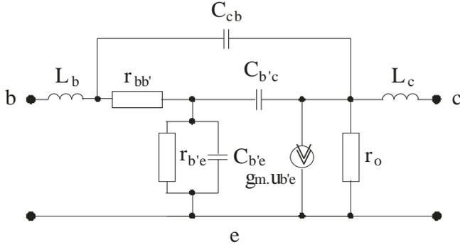
Fig. 2. Giacoletto high-frequency small-signal model for bipolar transistor
