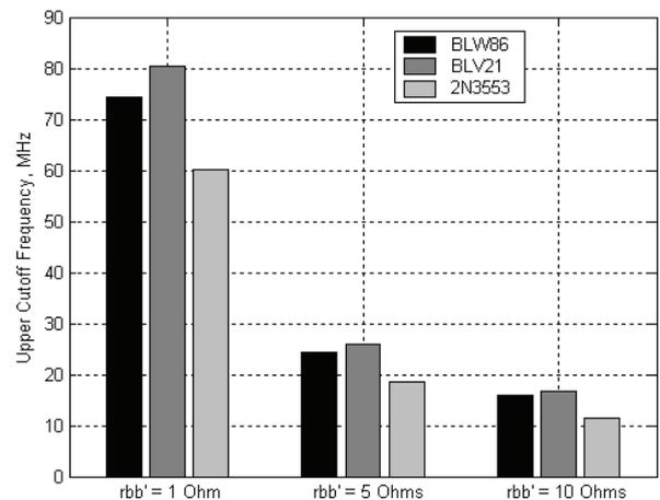
Fig. 6. Plot of upper cutoff frequency versus base – spreading resistance
