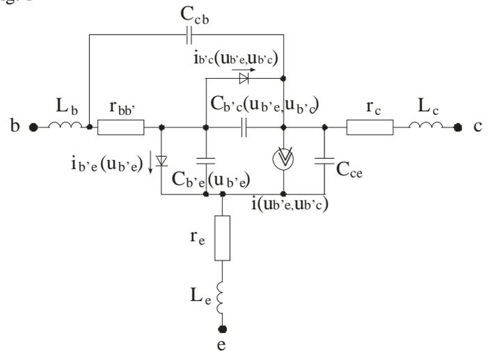
Fig.1. Nonlinear BJT model with extrinsic linear elements.
