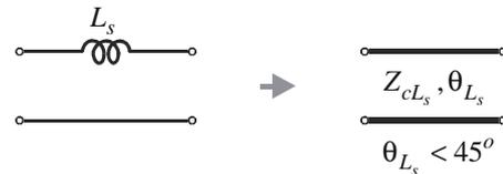
Fig.1. Synthesis of an inductance in series branch by transmission line of high characteristic impedance  $Z_{cL_s}$
