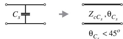
Fig.2. Synthesis of a capacitance in parallel branch by transmission line of low characteristic impedance  $Z_{cC_s}$
