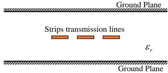
Fig. 5. Cross-section of three- strip conductors between two ground planes.
