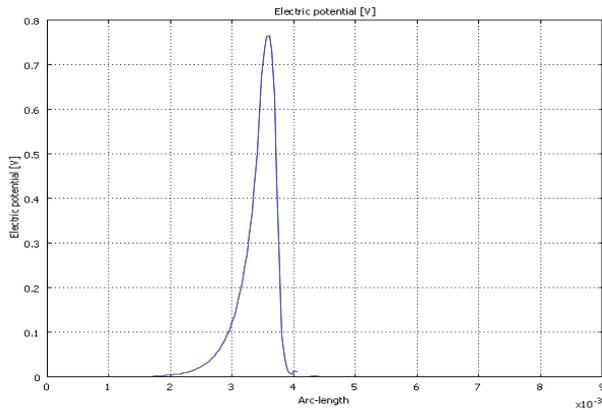
Fig. 8. Potential distribution of four- strip conductors between two ground planes along a line from (0, 0) to (8mm, 1mm).
