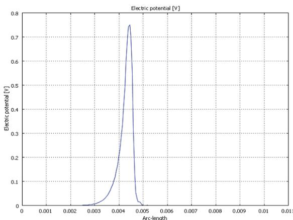
Fig. 10. Potential distribution of five- strip conductors between two ground planes along a line from (0, 0) to (10mm, 1mm).
