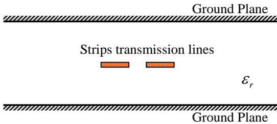
Fig. 3. Cross-section of two- strip conductors between two ground planes.
