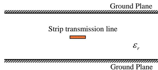
Fig. 1. Cross-section of single strip conductor between two ground planes.
