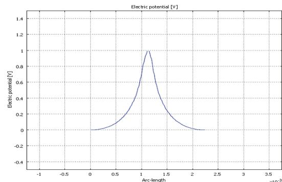
Fig. 2. Potential distribution of single strip conductor between two ground planes.along the line from (0, 0) to (2mm, 1mm).
