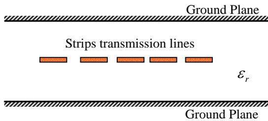
Fig. 9. Cross-section of five- strip conductors between two ground planes.
