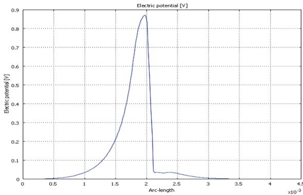
Fig. 4. Potential distribution of two-strip conductors between two ground planes along a line from (0, 0) to (4mm, 1mm).
