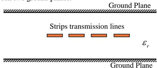
Fig. 7. Cross-section of four- strip conductors between two ground planes.
