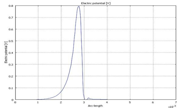
Fig. 6. Potential distribution of three- strip conductors between two ground planes along a line from (0, 0) to (6mm, 1mm).
