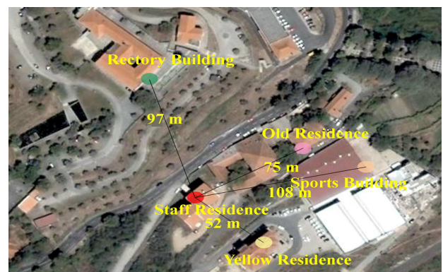
Fig.2- Point-to-multipoint wireless links for Pole II buildings.
