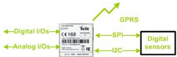
Figure 1. Localized data acquisition system
