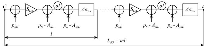
Fig. 2. Structural diagram of amplifying sections
