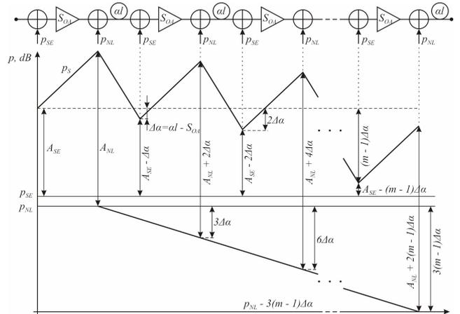
Fig. 4. Signal protectability diagram:  $A_{SE}$  – from spontaneous emitting,  $A_{NL}$  – from transient noise
