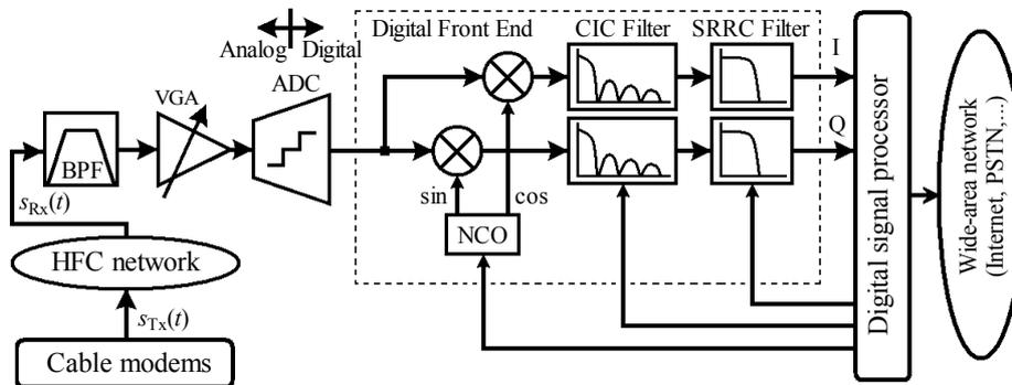
Fig. 3. Block diagram of the return path receiver
