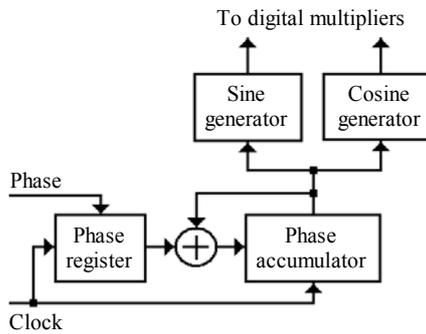
Fig. 4. Simplified block diagram of the quadrature NCO
