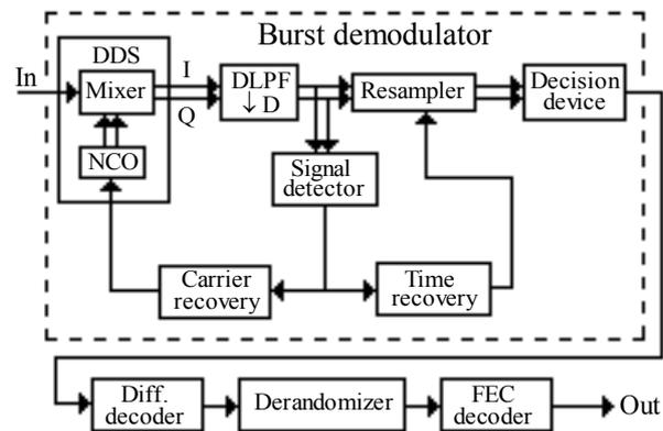
Fig. 1. Single module of the modular software headend
