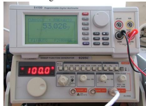
Fig. 10. Function Generator with the precision multimeter
