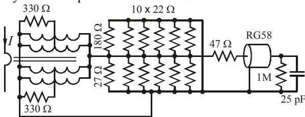
Fig. 3. Electric scheme of the current probe
