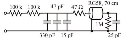
Fig. 5. Electric scheme of the flux probe
