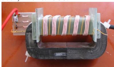
Fig. 12. Nanocrystalline material – Finemet, core F3CC016B
