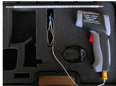
Fig. 9. Infrared thermometer with the thermocouple and the alcohol thermometer.
