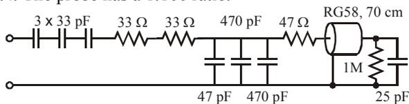
Fig. 4. Electric scheme of the voltage probe
