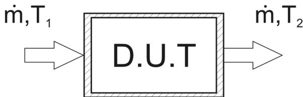
Fig. 7 Flow calorimeter principle
