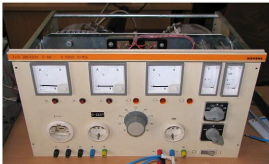
Fig.11 Power supply Siemens - 500V/10A
