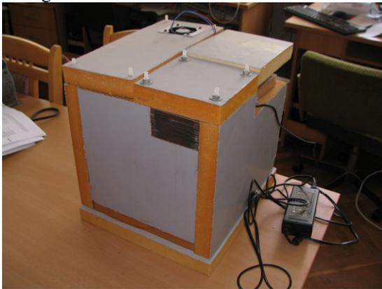
Fig. 8. Constructed calorimeter
