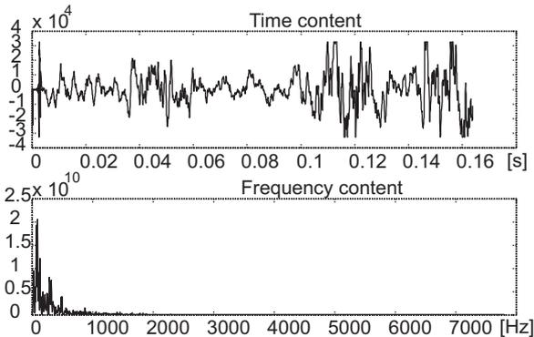
Fig. 2 – scratching noise signal time-flow and spectrum
