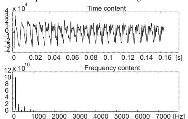
Fig. 6 – speech signal time-flow and spectrum
