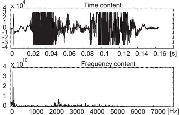
Fig. 8 – knocking signal time-flow and spectrum
