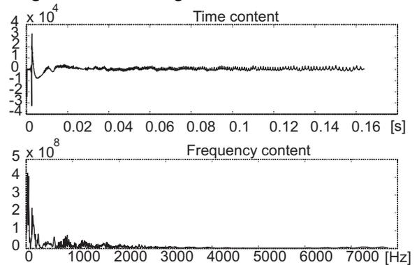
Fig. 4 – background noise signal time-flow and spectrum
