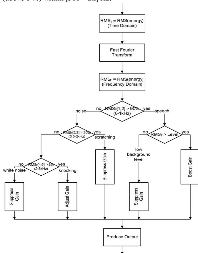
Fig. 11. – algorithm for recognizing types of noise
