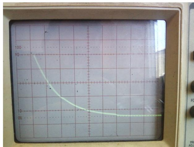
Fig. 3. Oscilloscope with fine adjusted time control settings to measure  $t_r$
