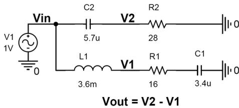
Fig. 9. Synthesized realizable transfer function
