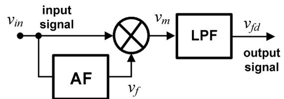
Fig. 3. Wideband Frequency Detector with an All Pass Filter
