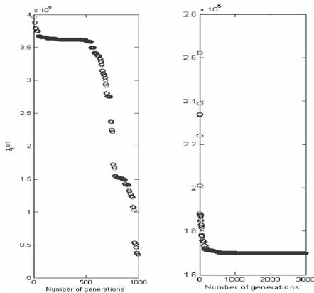
Fig. 11. Purpose function value during the GA synthesis procedure: experiment to obtain (7) (left) and experiment to obtain (5) (right)
