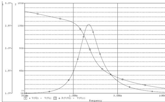
Fig. 10. Magnitude and phase response of the Synthesized Circuit
