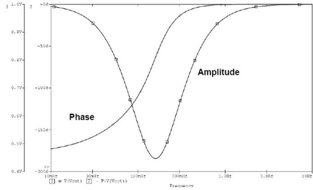
Fig. 6. Magnitude and phase responses of the proposed non-minimum phase filter
