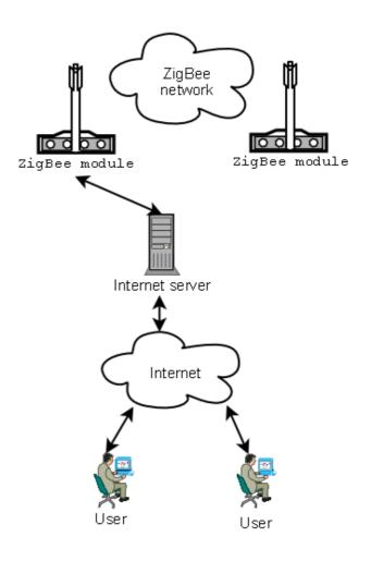
Fig. 1. The block diagram of the Internet-Zigbee based system model for measurement and control
