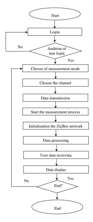
Fig. 2. The algorithm implemented for processes in the Internet-Zigbee based system model for measurement and control
