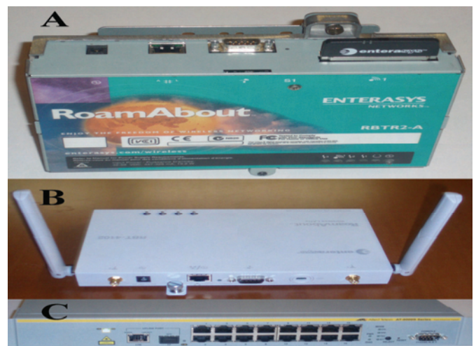
Fig. 1- Access Points (A), (B) [12] and switch (C) [13].
