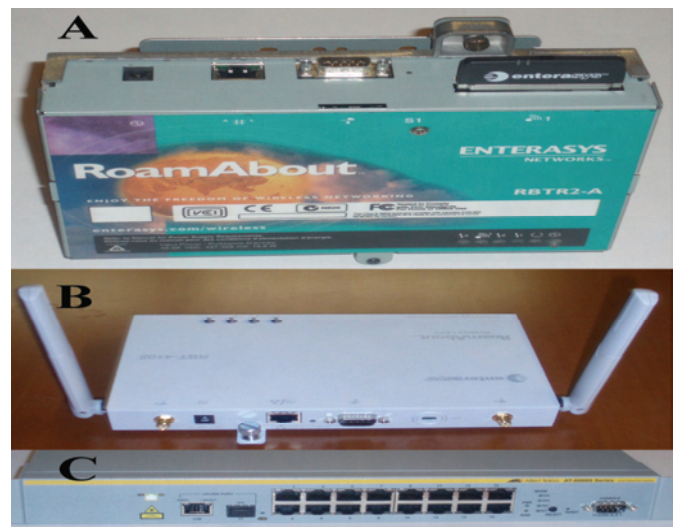
Fig. 1- Access Points (A), (B) [12] and switch (C) [13].
