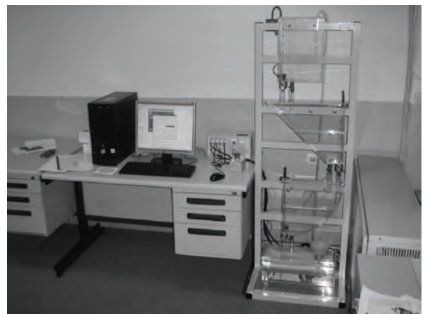
Fig. 4. Multitank hydraulic system
