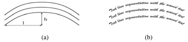
Fig.5. (a) Waved text referent line shape definition ( h and l are parameters), (b) Waved multi-line text sample
