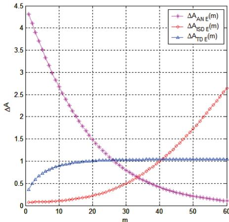
Fig. 4. Losses due to transient, intersymbol distortions and additive noises as function of the number of amplifying sections
