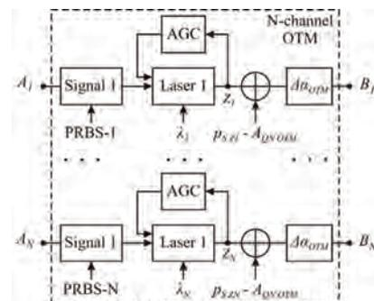
Fig. 2. Structural diagram of optical transmission module
