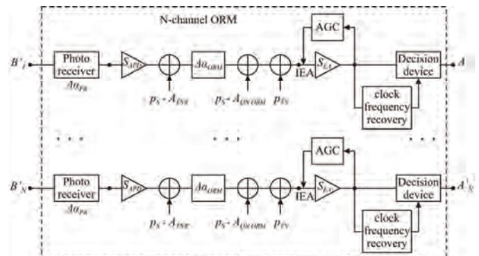
Fig. 3. Structural diagram of optical reception module
