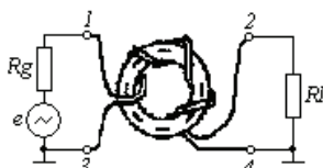
Fig. 1. Transmission Line Transformer
