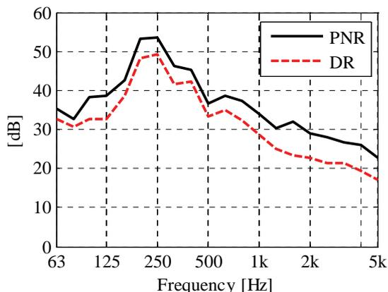
Fig. 3. PNR of the receiver room impulse response together with DR of the corresponding decay curves
