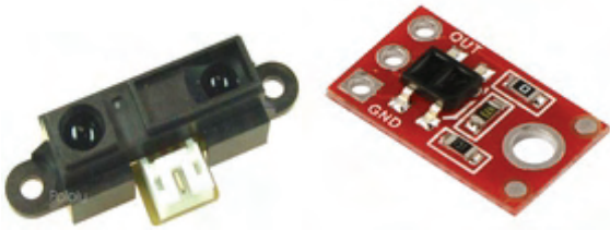
Fig 3. Distance and surface colour sensors
