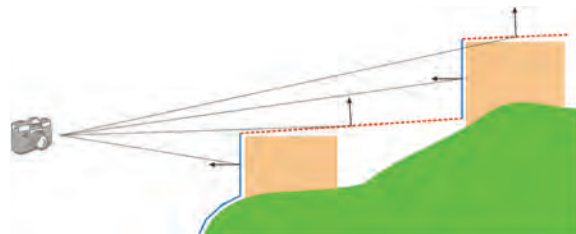
Fig. 3. Elimination of false visible surfaces using the orientation test
