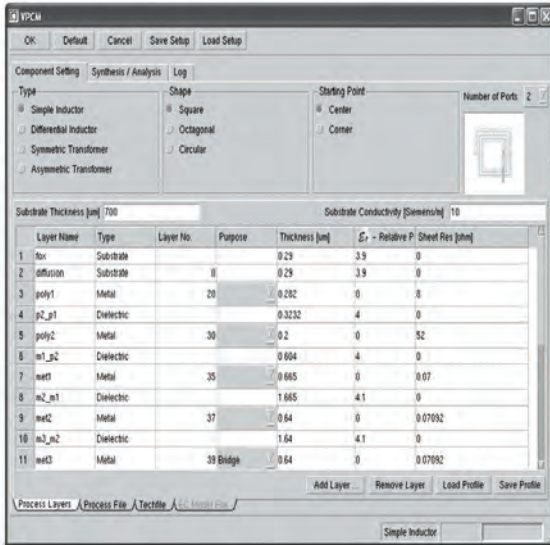
Fig. 3. Window from CADENCE tool “Virtuoso Passive Component Designer”.
