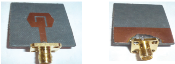
Fig. 2. Antenna 2: Hexagonal monopole antenna with asymmetrical U-slot (a) Antenna geometry (b) Photograph
