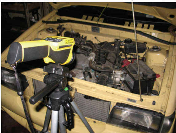
Fig. 12 Application of thermal camera in diagnostics of system for gas
