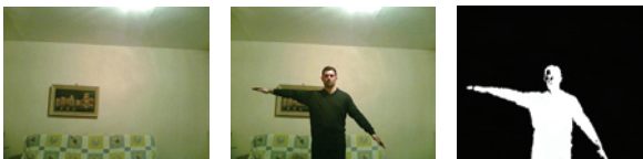
Fig. 5. Image differencing with reference image. From left to right: reference image, input image, output image
