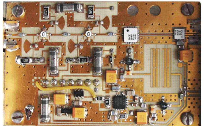
Fig. 4 Photo of the laboratory model of the receiver
