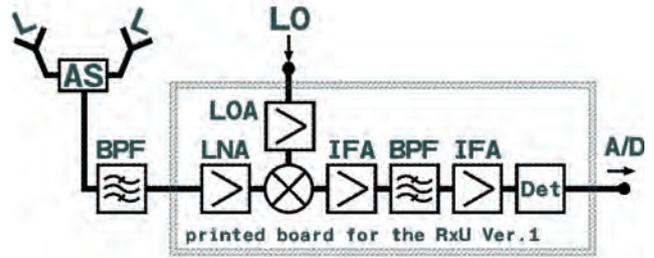
Fig. 3. A block- scheme of the laboratory model of the receiver
