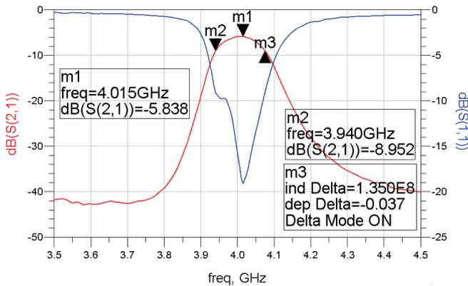
Fig.8 Measured characteristics of the IF band-pass filter
