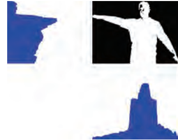
Fig. 6. Horizontal and vertical histogram of the detected human's body
