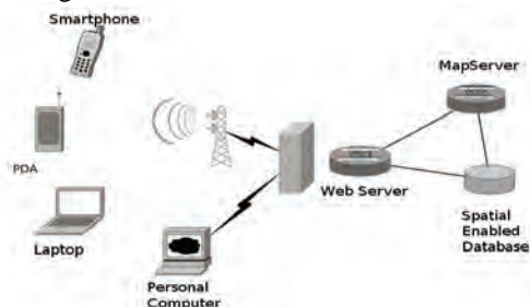
Fig. 2: Overview of the architecture, main components and typical usage of the application
