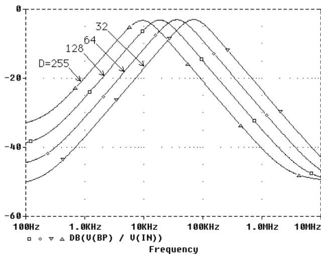
Fig. 5. Simulated frequency responses of the BP filter when the digital code  $D$  is varied.
