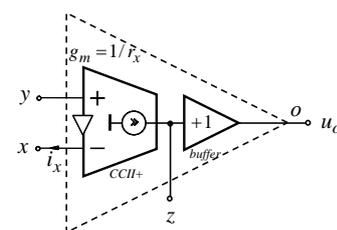
Fig. 1a. Symbol of a four-terminal CFOA.
