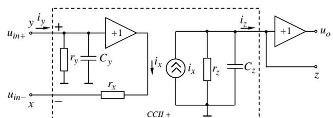
Fig. 1b. Linear macro-model of a four-terminal CFOA.
