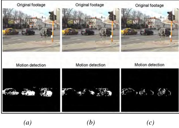
Fig. 1. Temporal Averaging method executed for three amounts of \alpha , \alpha = 0.01 (a); \alpha = 0.1 (b); \alpha = 0.8 (c)
