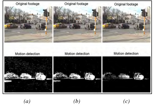
Fig. 4. Mixture of Gaussians background subtraction method executed for three amounts of T , T = 0.25 (a); T = 0.35 (b); T = 0.5 (c)
