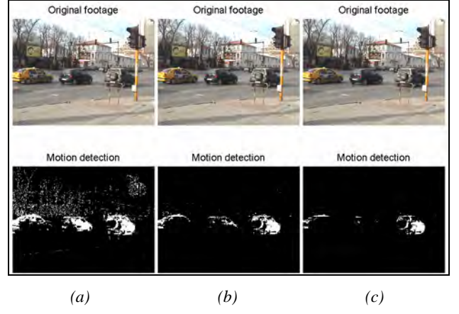
Fig. 3. \Sigma - \Delta background modeling executed for three amounts of C , C = 1 (a); C = 5 (b); C = 20 (c)
