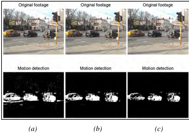
Fig. 2. Temporal Averaging method executed for three amounts of T , T = 25 (a); T = 40 (b); T = 55 (c)
