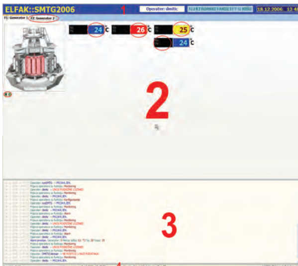
Fig. 2. Temperature monitoring screen
