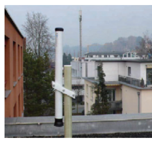
Fig. 8. Sensor located outdoor on the roof.
