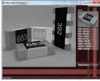
Fig. 1. Animation module for the demonstration of surface mount components: Part I - resistors.
