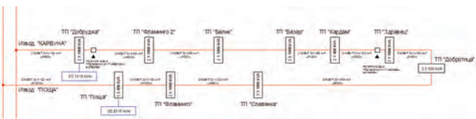
Fig. 3. Albena Resort Feeder "C" 20 kV
