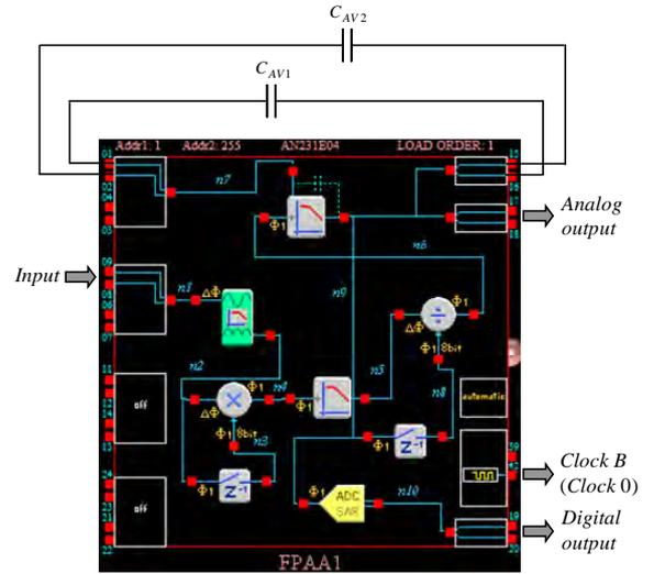
Fig. 3. FPAA configuration of RMS-to-DC converter from Fig. 1.
