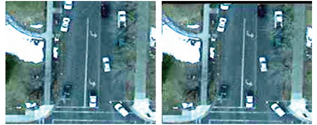
Fig.3 The frame from aerial video and its global motion removed version
