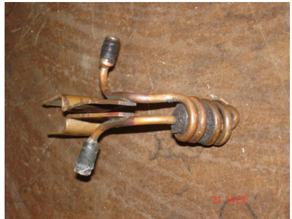
Fig. 9. An inductor used for hardening of internal cylindrical surfaces of steel sleeves
