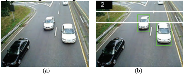
Fig. 5: original frame (a), counting area with counter of number of vehicles currently present in it (b)
