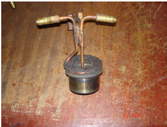
Fig. 8. A typical system inductor-detail used in Pomorie PLC
