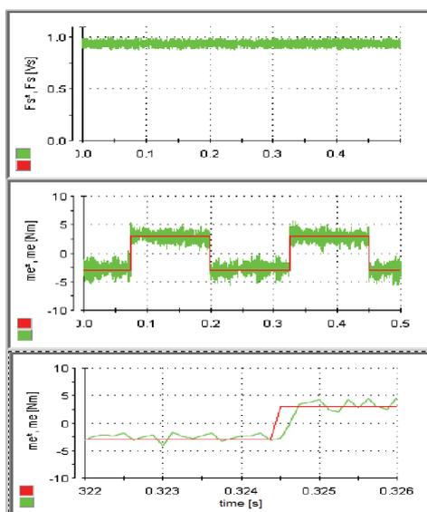
Fig. 8. DTC with twelve sector switching technique
