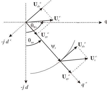
Fig. 4. Stator flux vector in synchronous reference frame
