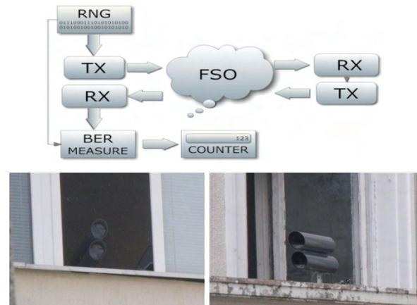
Fig. 1. Block scheme and real pictures of FSO
