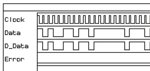
Fig. 7. Computer simulation without errors
