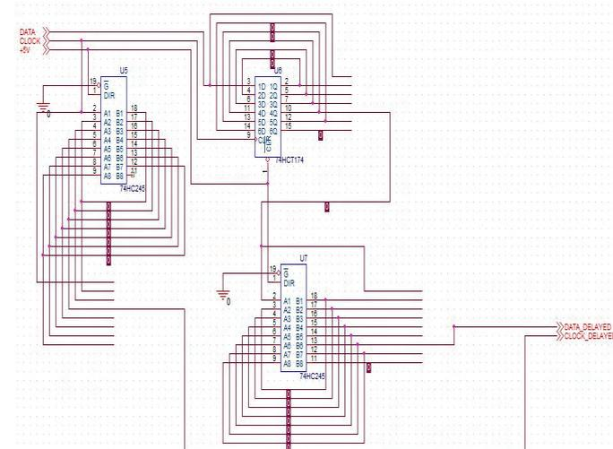
Fig. 4. Principal realization of scheme for long delays
