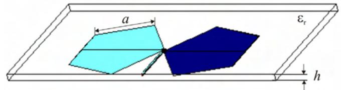
Fig.1. Printed pentagonal dipole
