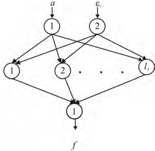
Fig. 4. Neural model of printed pentagonal dipole
