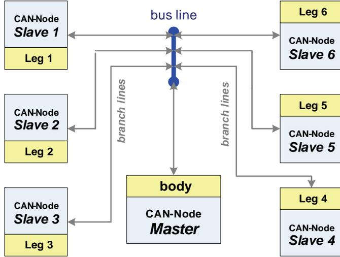
Fig.2. The Master in connection with all six slaves
