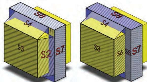
Fig.1 Equivalent surfaces of an EE transformer, left for radiation; right for convection
