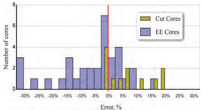
Fig.4 Distribution of the error from using one  $k_A$ :  $T_w=100^\circ\text{C}$  (EE cores),  $T_w=120^\circ\text{C}$  (cut cores),  $T_{\text{amb}}=30^\circ\text{C}$ ,  $v=0\text{m/s}$ ,  $\varepsilon_T=0,96$ .
