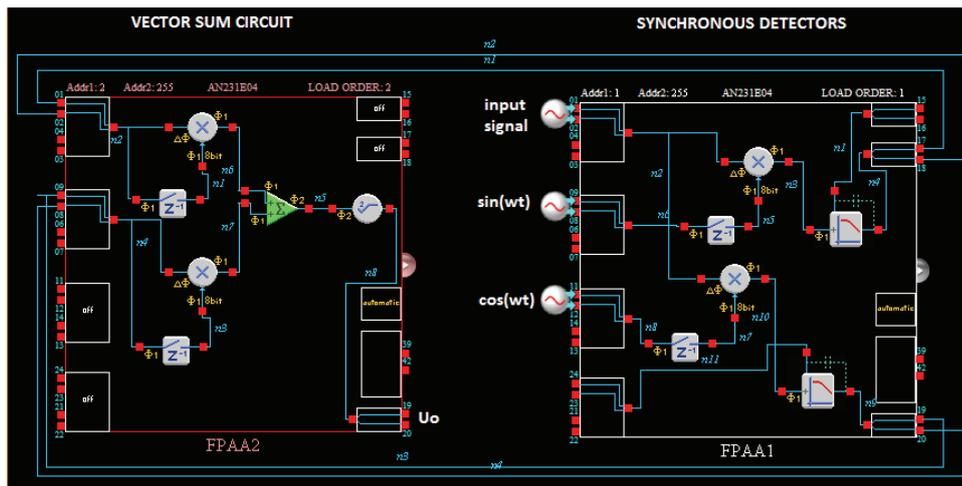
Fig. 2. FPAAs configuration of synchronous detector from Fig. 1.
