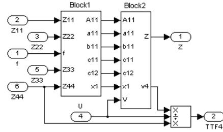
Fig. 2. Matlab/Simulink model of the piezoceramic ring
