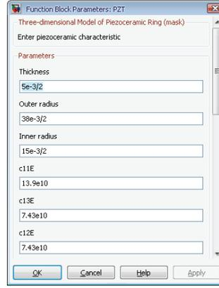
Fig. 6. Mask dialog block for the enter piezoceramic ring parameters
