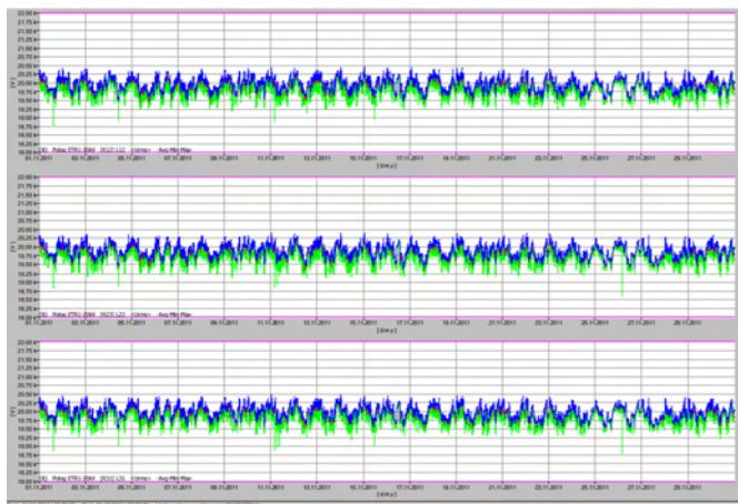
Fig. 1. Voltage magnitude variations at 20 kV level of TS Polog 110/20 kV/kV
