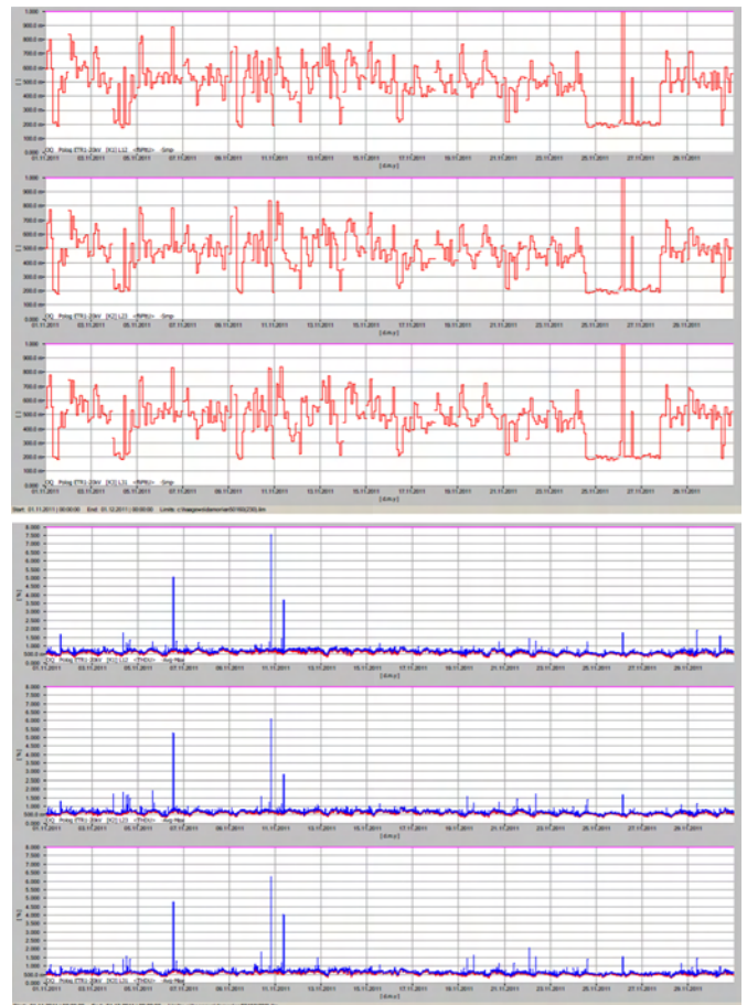
Fig. 3. Flicker severity and total harmonic distortion factor at 20 kV level of TS Polog 110/20 kV/kV
