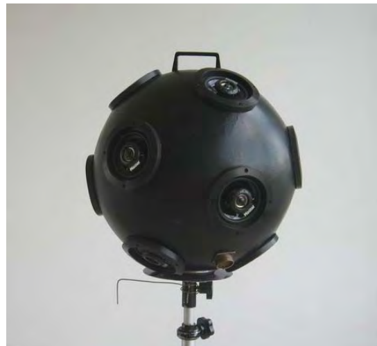
Fig. 1. Sound source with independent elements (loudspeakers) in the form of a dodecahedron
